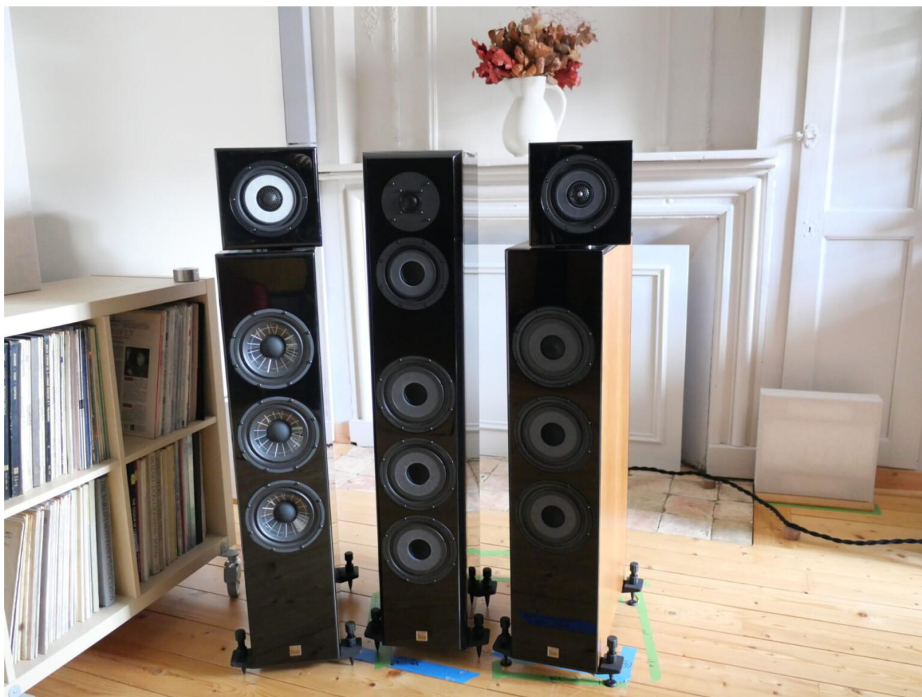
The three Vienna Acoustics speakers again – emphasising the differences in cabinet construction and driver technology, but also the similarities in size and overall topology.
