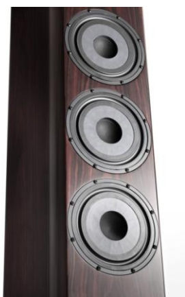
A close up of the composite cone drivers: note the flat diaphragm, radial ribs for stiffness and the large diameter, inverted central fabric dome.
